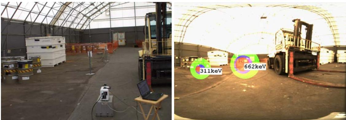
Figure 10 Compton image of the waste drums contributing to the 311 and 662 keV gamma-ray lines in the spectrum shown in Figure 7. Passive imaging allows for the accurate characterization of waste containers, reducing possible interference from adjacent source of radioactivity.
