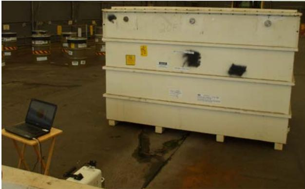
Figure 6 GeGI with PC interface (lower left) was positioned to measure a waste bin at the SRS storage facility.
