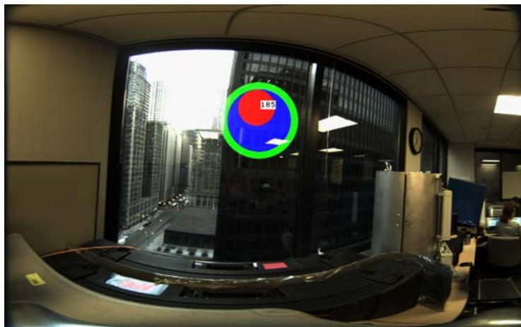
Figure 5 Compton image of highly enrichment uranium (~100 grams of material) located in a building approximately 28 m away. The 186 keV gamma ray from  $^{235}\text{U}$  was detected spectrally in 15 minutes and localized within 40 minutes.
