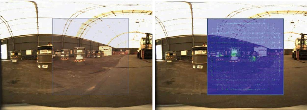
Figure 9 Pinhole image at 59.9 keV, clearly showing the 59.5 keV peak in Figure 7 results from the contribution of three individual waste drums.
