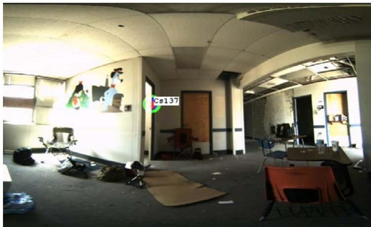
Figure 4 A Compton image of a  $^{137}\text{Cs}$  source located in an adjacent room. The imaging capability of GeGI can be used to verify the non-nuclear nature of a facility.
