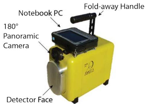
Figure 1 The Germanium Gamma-Ray Imager (GeGI) with attached PC for instrument control and data storage. The 180° panoramic camera provides an optical photograph to overlap on the Compton and Pinhole images.
