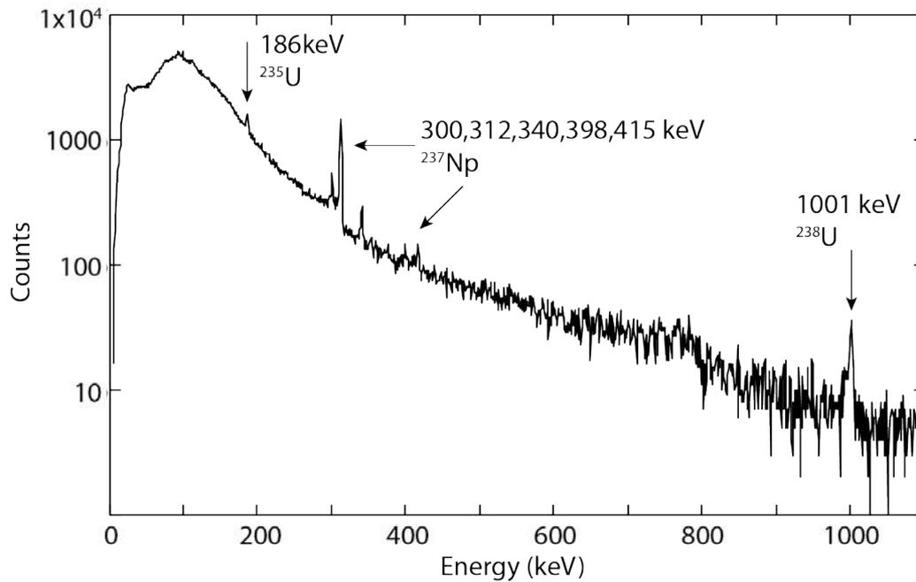
Figure 2 Spectrum taken at the Paducah Uranium Gaseous Diffusion Plant indicating the presence of  $^{237}\text{Np}$  contamination of uranium gaseous-diffusion lines.
