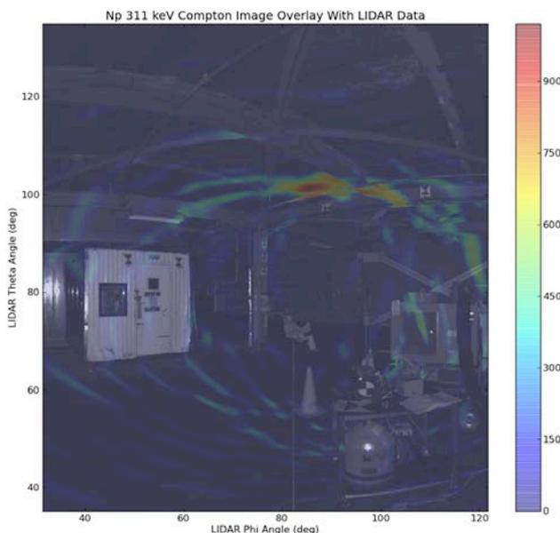
Figure 3 Compton image localizing the pipe with  $^{237}\text{Np}$  contamination. This information can be used to quantify the amount of material and for cleanup efforts.
