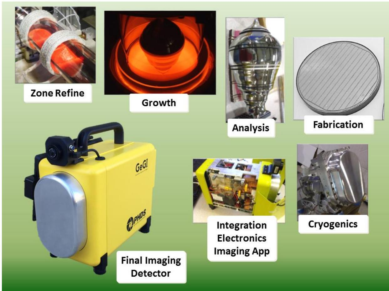
Figure 3. From raw materials through radiological answer, the manufacturing process starts with germanium material refinement, continuing with crystal growth, detector fabrication and system integration to complete the Germanium Gamma-ray Imaging (GeGI) detector system.
