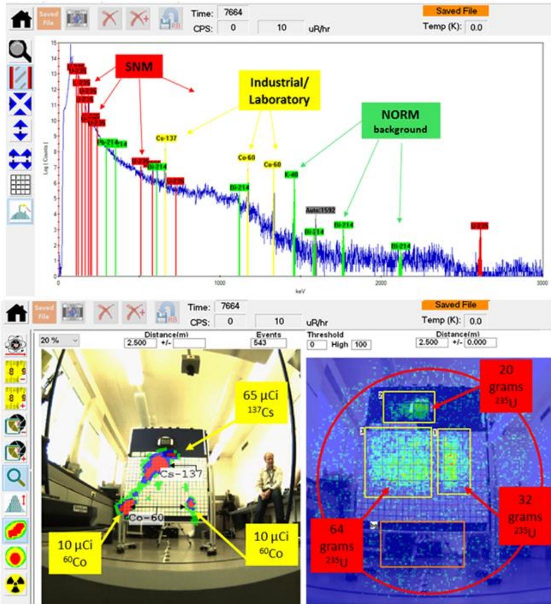
Figure 7. A simultaneous Compton and Pinhole Image. The Compton imaging locates, identifies and quantifies  $^{60}\text{Co}$  and  $^{137}\text{Cs}$  sources while pinhole imaging showed detailed regions (and missing regions!) of an enriched  $^{235}\text{U}$  fuel assembly.
