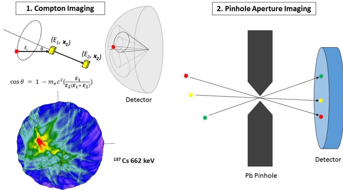
Figure 4. Compton Imaging and Pinhole Aperture Imaging are both simultaneously accommodated by the Germanium Gamma-ray Imaging Detector. Compton Imaging is well suited to high sensitivity search while pinhole imaging makes highly detailed object images including shape and substructure information.
