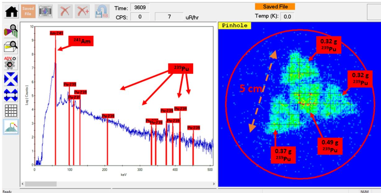
Figure 6. The energy spectrum and pinhole-aperture image from the triangular  $^{239}\text{Pu}$  object. The gamma-ray image reveals the object to be made up of four smaller triangular chambers each containing a relatively uniform planar distribution of  $^{239}\text{Pu}$  quantified as shown.
