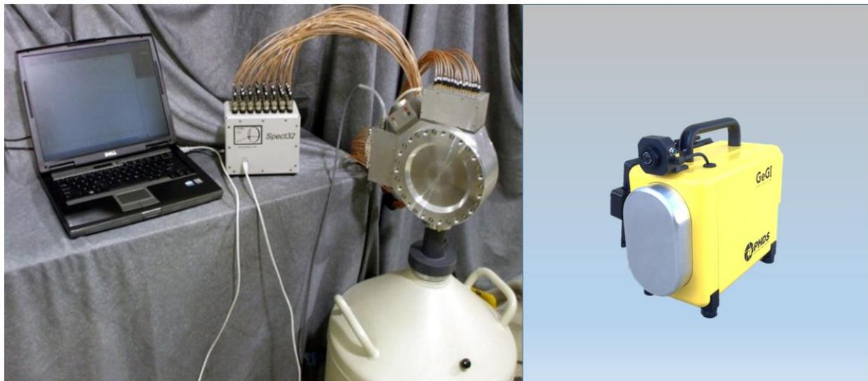
Figure 2. On the left a laboratory imaging detector developed for nuclear-physics research relies on liquid nitrogen for cryogenic operation ( $\sim 150$  lbs.). On the right, the 28 lb. GeGI has a detector of the same size with all electronics and a Stirling cycle mechanical cooler contained inside the yellow box.
