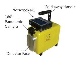
Figure 1 The Germanium Gamma-Ray Imager (GeGI) with attached PC for instrument control and data storage. The 180° panoramic camera provides an optical photograph to overlap on the Compton and Pinhole images.
