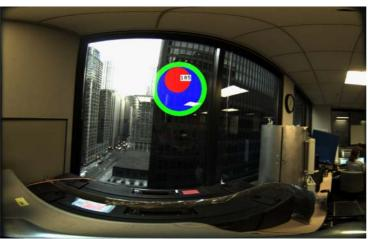
Figure 5 Compton image of highly enrichment uranium (~100 grams of material) located in a building approximately 28 m away. The 186 keV gamma ray from <sup>235</sup>U was detected spectrally in 15 minutes and localized within 40 minutes.
