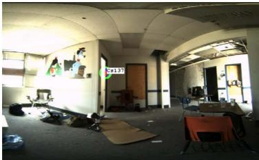
Figure 4 A Compton image of a <sup>137</sup>Cs source located in an adjacent room. The imaging capability of GeGI can be used to verify the non-nuclear nature of a facility.
