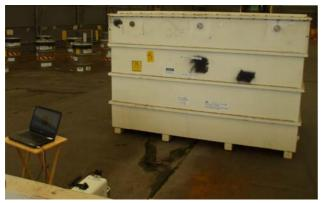
Figure 6 GeGI with PC interface (lower left) was positioned to measure a waste bin at the SRS storage facility.
