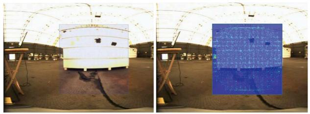
Figure 8 Pinhole image taken of the waste bin shown in Figure 7 at 59.5 keV. This gammaray line is visible in the spectrum (Figure 7, left) but was found to be from a waste drum located behind the bin, not the bin itself.
