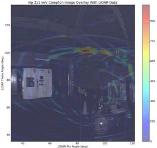
Figure 3 Compton image localizing the pipe with <sup>237</sup>Np contamination. This information can be used to quantify the amount of material and for cleanup efforts.
