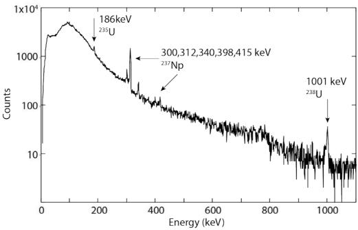
Figure 2 Spectrum taken at the Paducah Uranium Gaseous Diffusion Plant indicating the presence of <sup>237</sup>Np contamination of uranium gaseous-diffusion lines.
