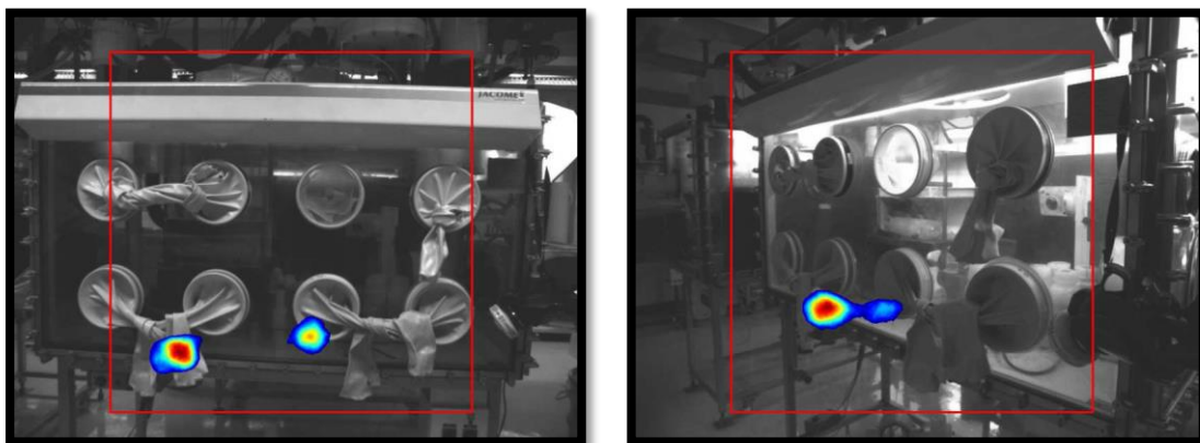
Figure 133. System6 gamma-ray images from the glovebox high-activity scenario, where two hot spots are localized.
