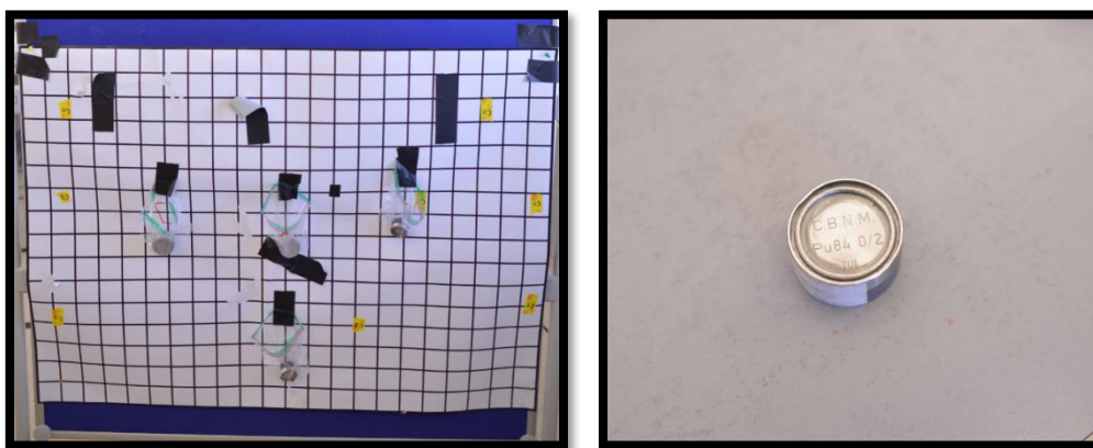
Figure 108. E7M32 – geometry of measurements (left), CBNM Pu84 source geometry (right)
