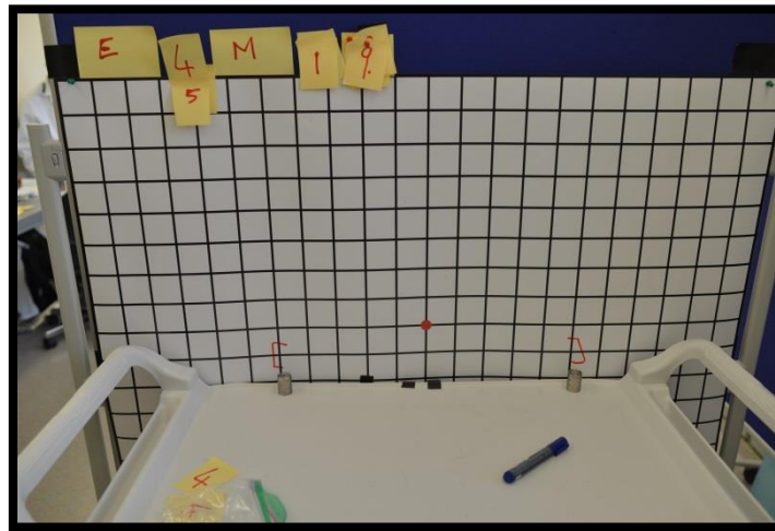
Figure 74. Illustration of the geometry of angular resolution measurements. Distance between two Am-Li sources is 50 cm.
