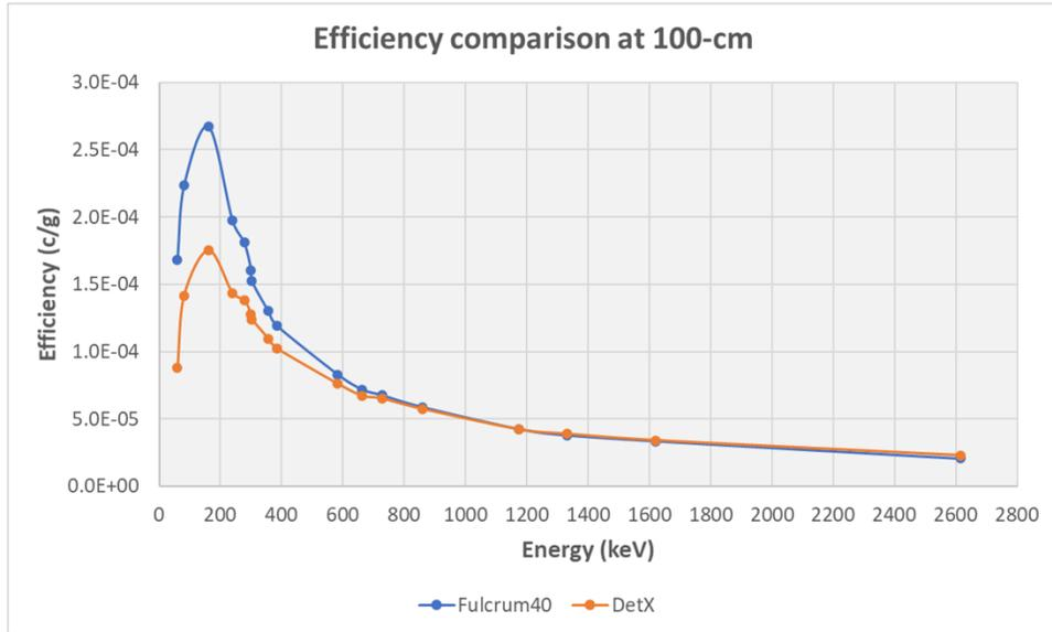
Figure 2. Average gamma efficiency comparison at 100-cm.
