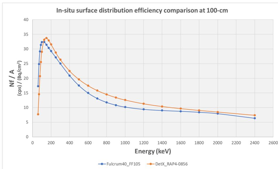
**Figure 5. In-situ surface distribution efficiency comparison.**
