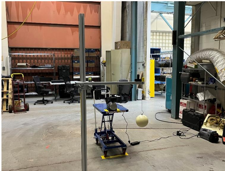
**Figure 6. Fulcrum40h neutron efficiency measurement in progress.**
