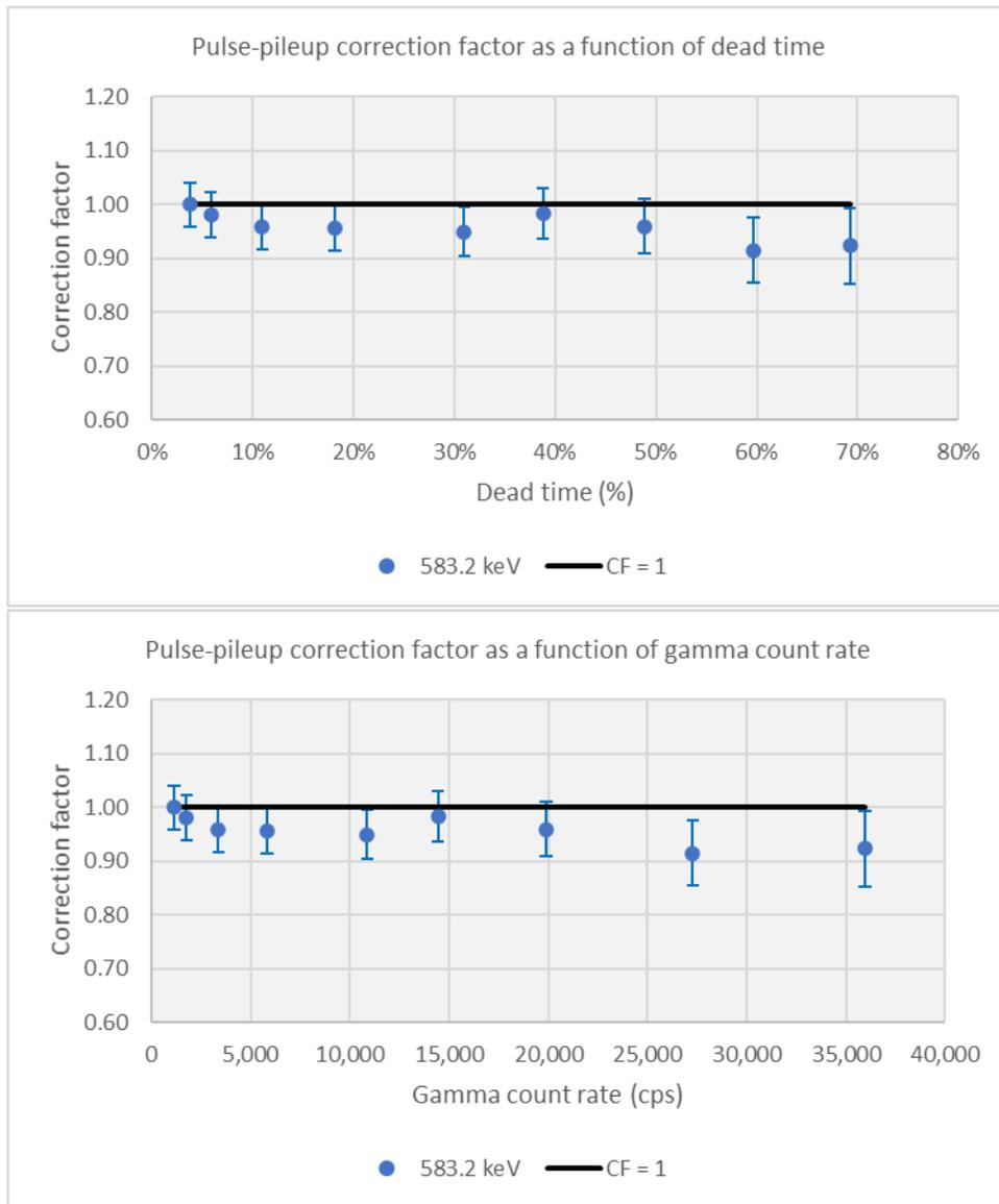
**Figure 9. Detective-X (21180856) pulse-pileup correction factor at 583.2 keV as a function of dead time and gamma count rate.**
