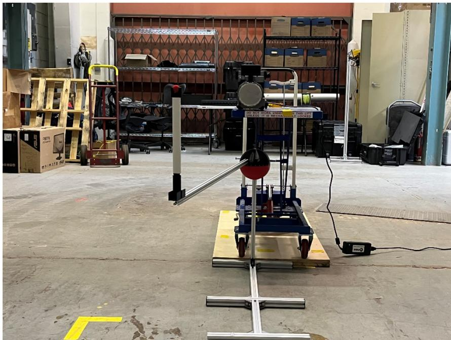
Figure 4. Fulcrum40h in-situ angular response measurement in progress.
