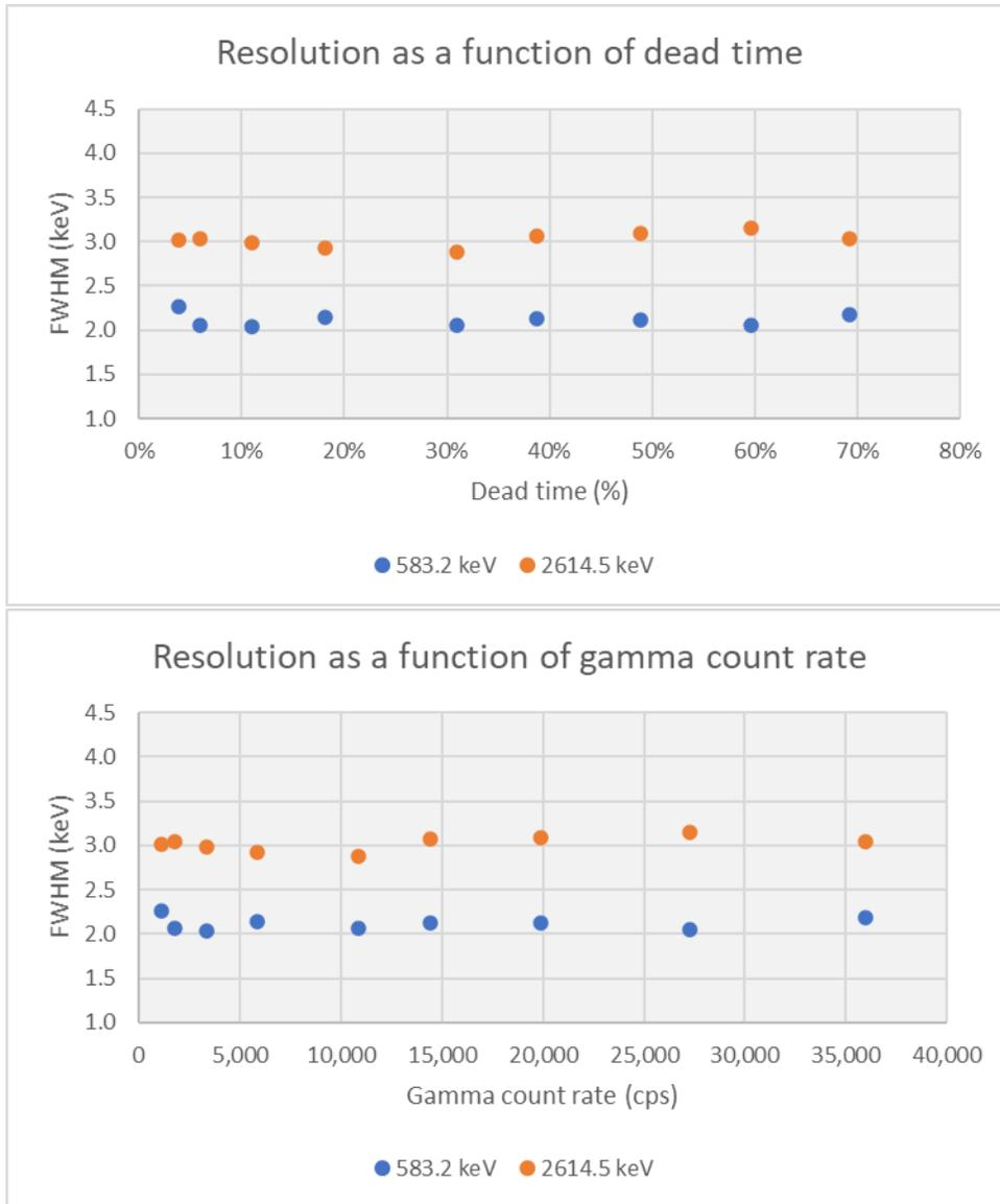
Figure 11. Detective-X (21180856) resolution as a function of dead time and gamma count rate.
