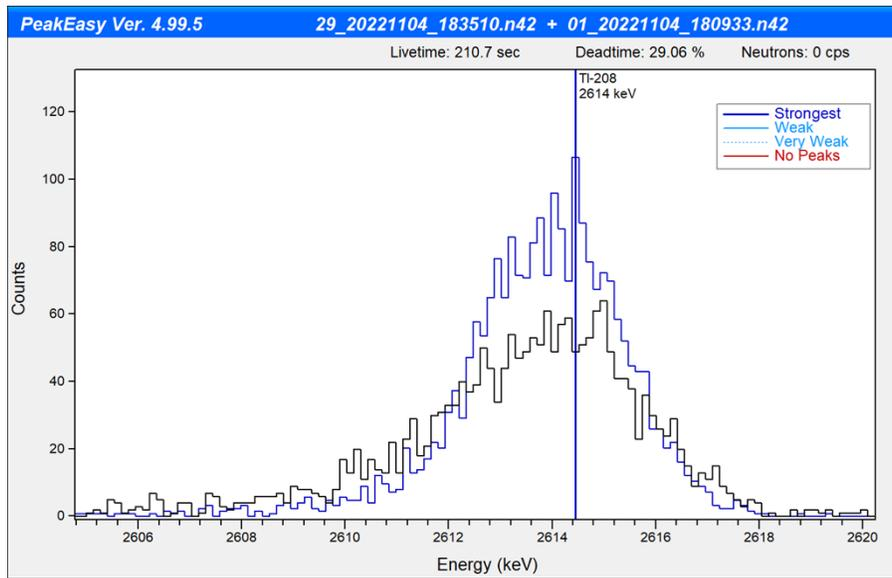
**Figure 12. Fulcrum40h (FF105) 2614.5 keV peak resolution measured at minimal dead time (blue) and  $\approx 30\%$  dead time  $\approx 37,000$  cps (black). Linear scale.**
