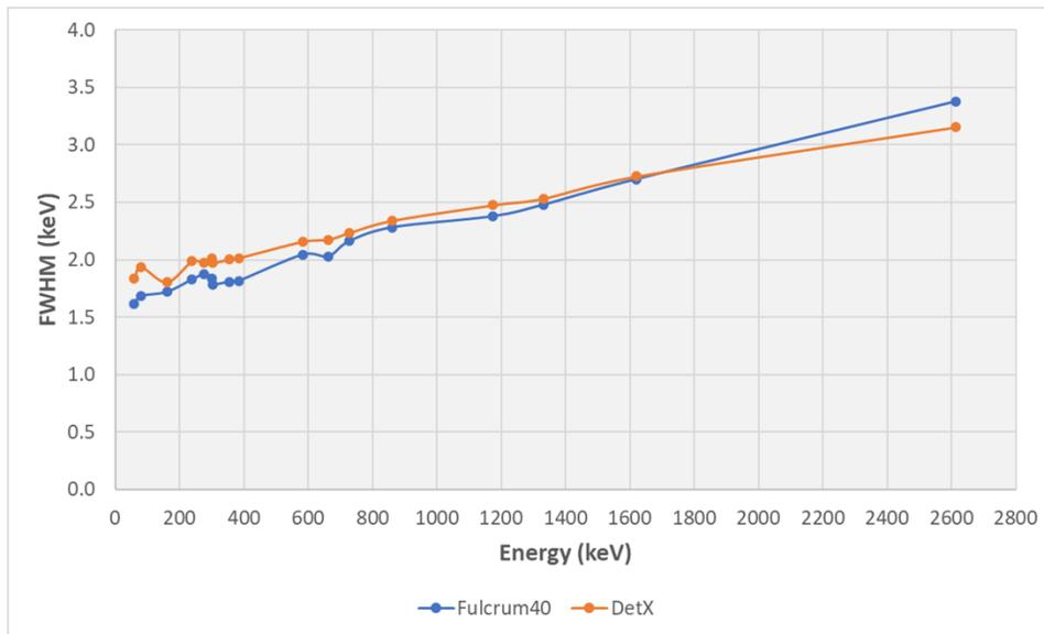
Figure 3. Average gamma resolution comparison.
