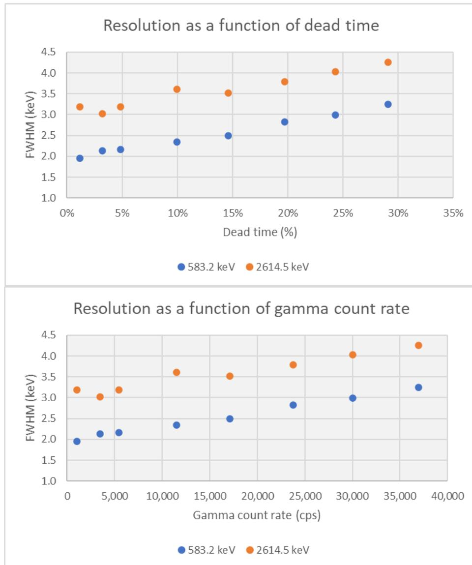
Figure 10. Fulcrum40h (FF105) resolution as a function of dead time and gamma count rate.
