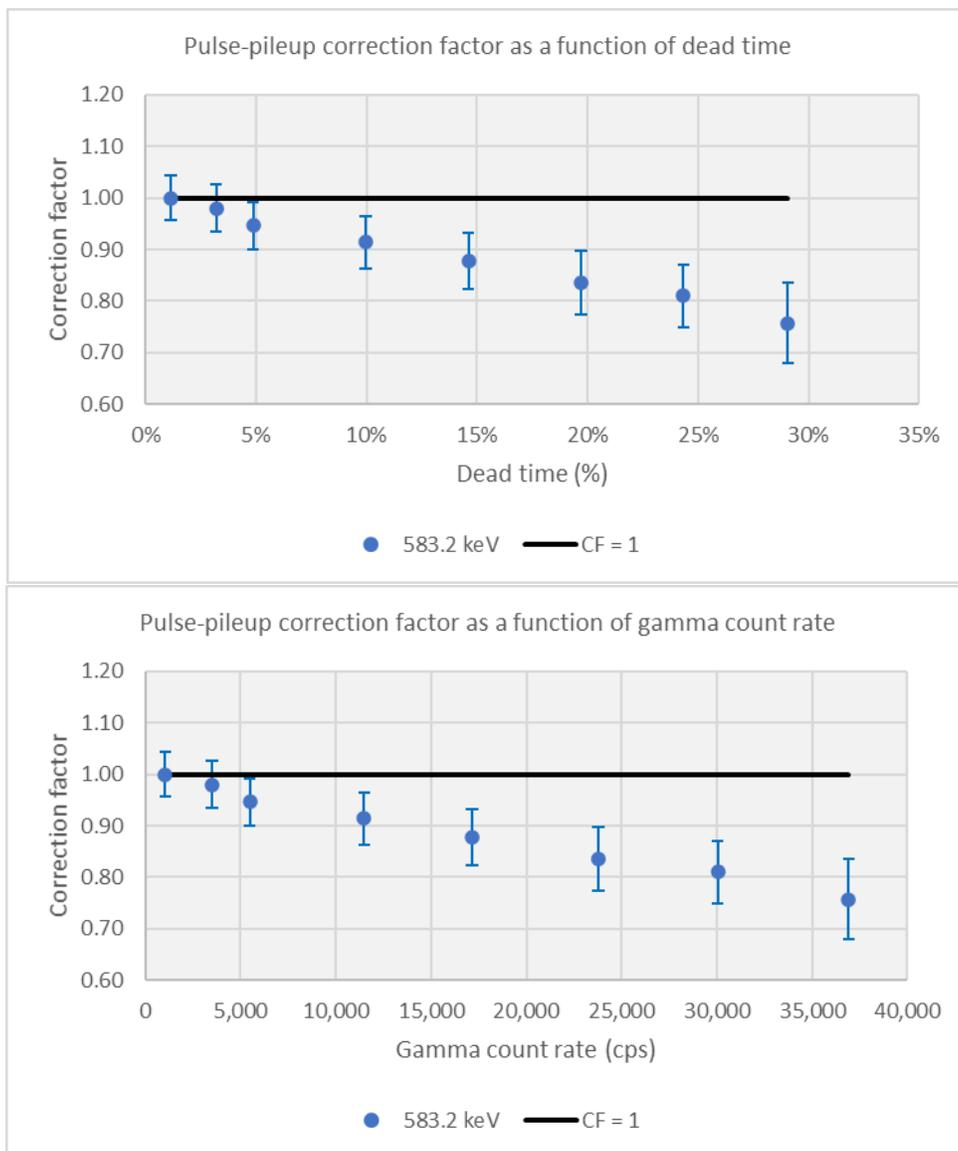
**Figure 8. Fulcrum40h (FF105) pulse-pileup correction factor at 583.2 keV as a function of dead time and gamma count rate.**
