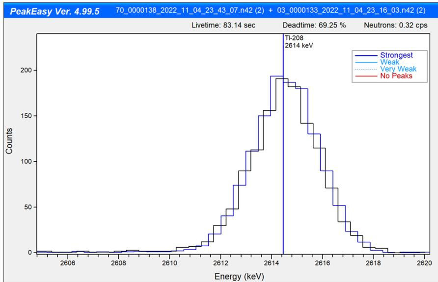
**Figure 13. Detective-X (21180856) 2614.5 keV peak resolution measured at minimal dead time (blue) and  $\approx 70\%$  dead time  $\approx 36,000$  cps (black). Linear scale.**
