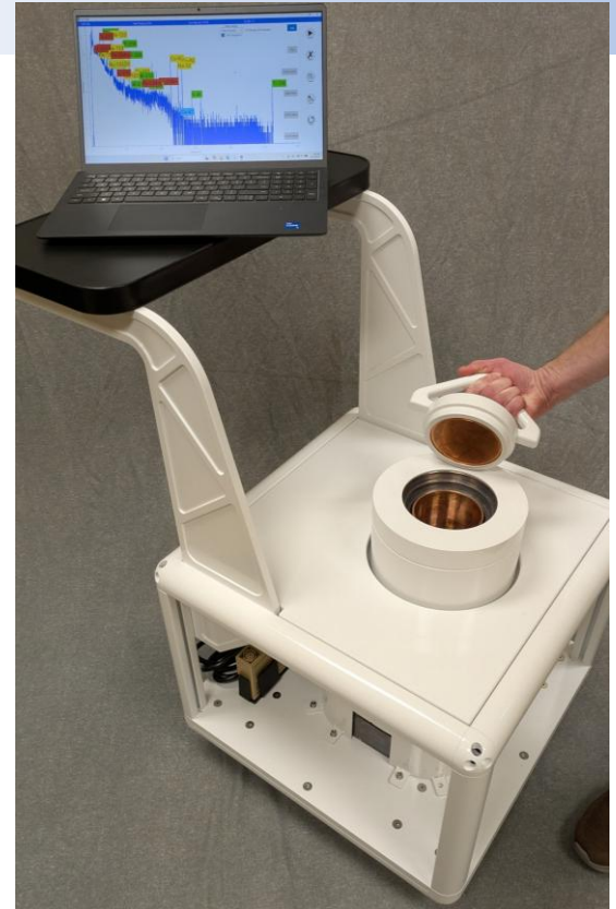
Manual Laboratory Operation of Fulcrum-L HPGe Detector for Shielded Radio Assay Measurements
